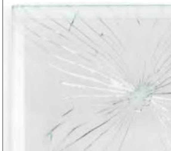
GSD Doublemirror - example of breakage
